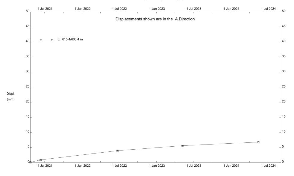
C007; H16:30; Kenilworth Lake Slide, Inclinometer SI21-C07-01
