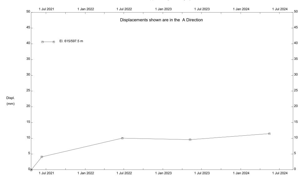
C007; H16:30; Kenilworth Lake Slide, Inclinometer Sl21-C07-02
