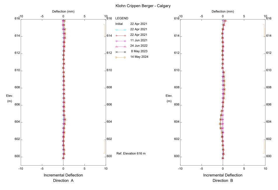
C007; H16:30; Kenilworth Lake Slide, Inclinometer Sl21-C07-01
