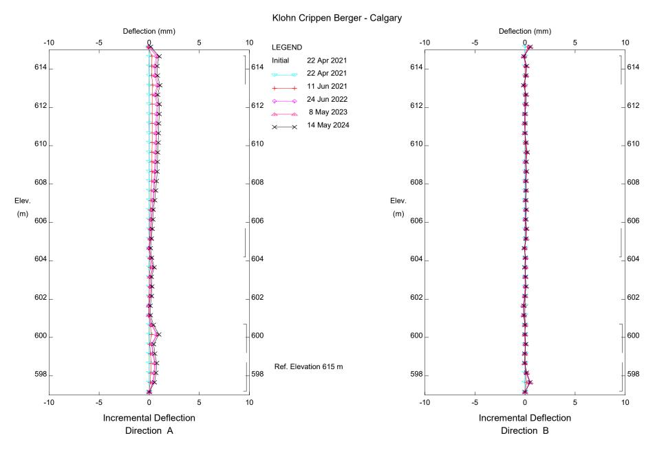
C007; H16:30; Kenilworth Lake Slide, Inclinometer Sl21-C07-03
