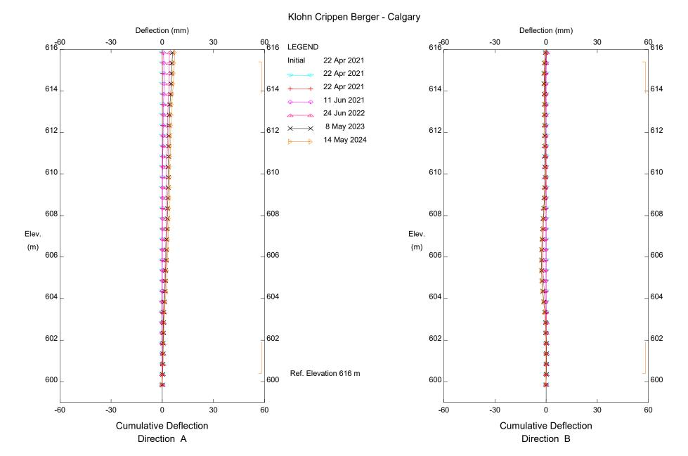
C007; H16:30; Kenilworth Lake Slide, Inclinometer Sl21-C07-01
