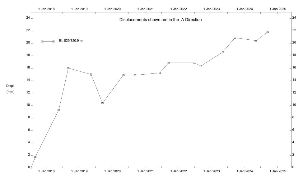
C067; H21:14, Kneehill Creek Slide, Inclinometer SI16-02
