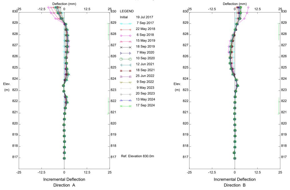
C067; H21:14, Kneehill Creek Slide, Inclinometer SI16-02
