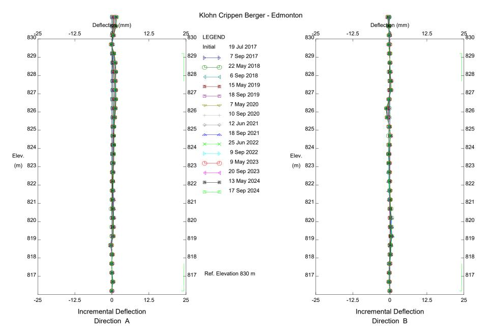
C067; H21:14, Kneehill Creek Slide, Inclinometer SI17-C67-01
