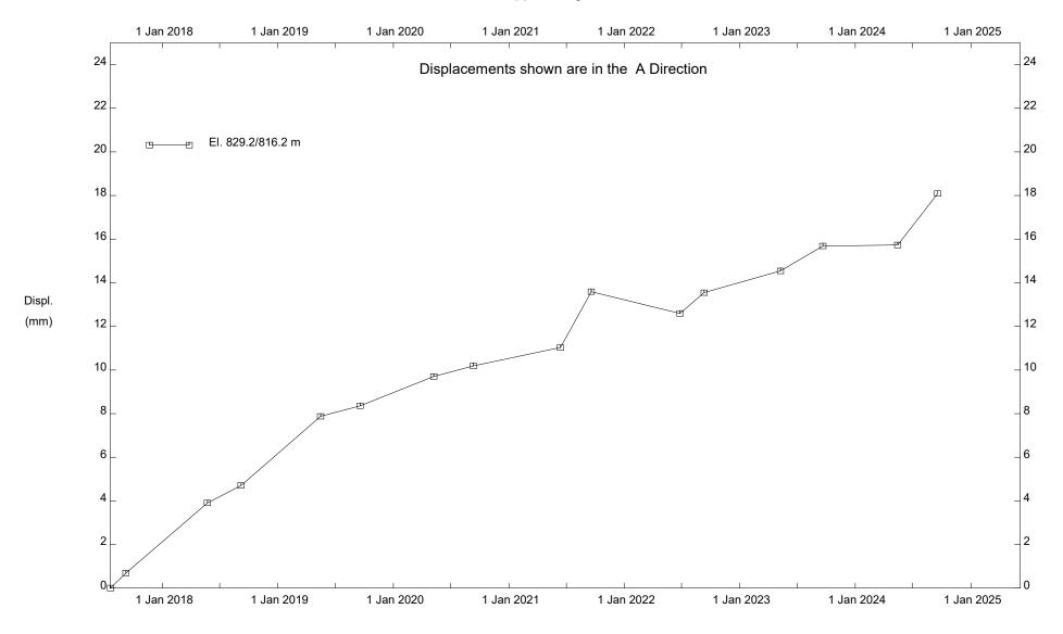
C067; H21:14, Kneehill Creek Slide, Inclinometer SI17-C67-01
