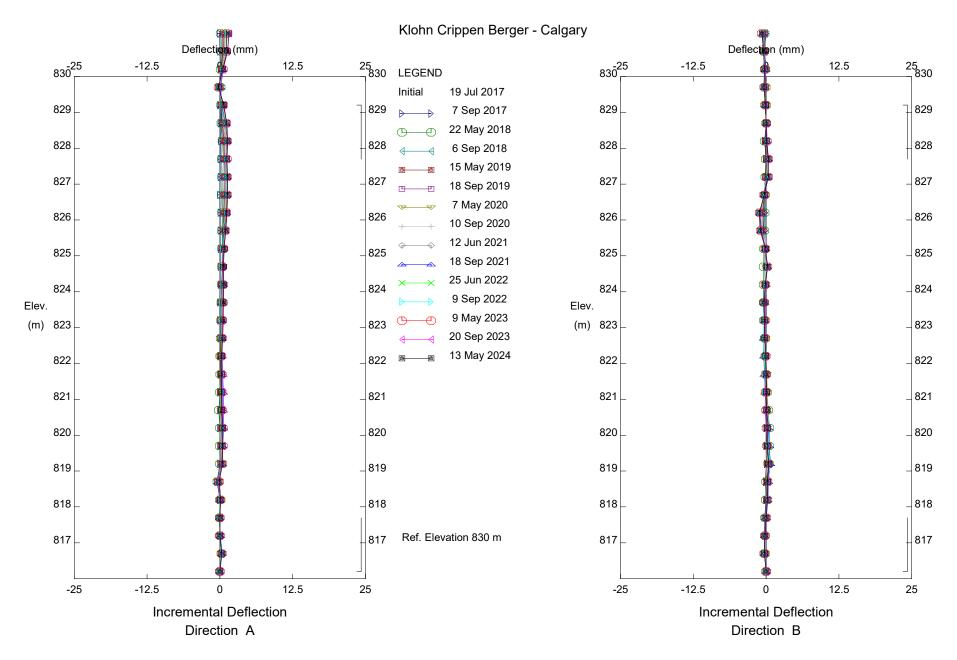
C067; H21:14, Kneehill Creek Slide, Inclinometer SI17-C67-01
