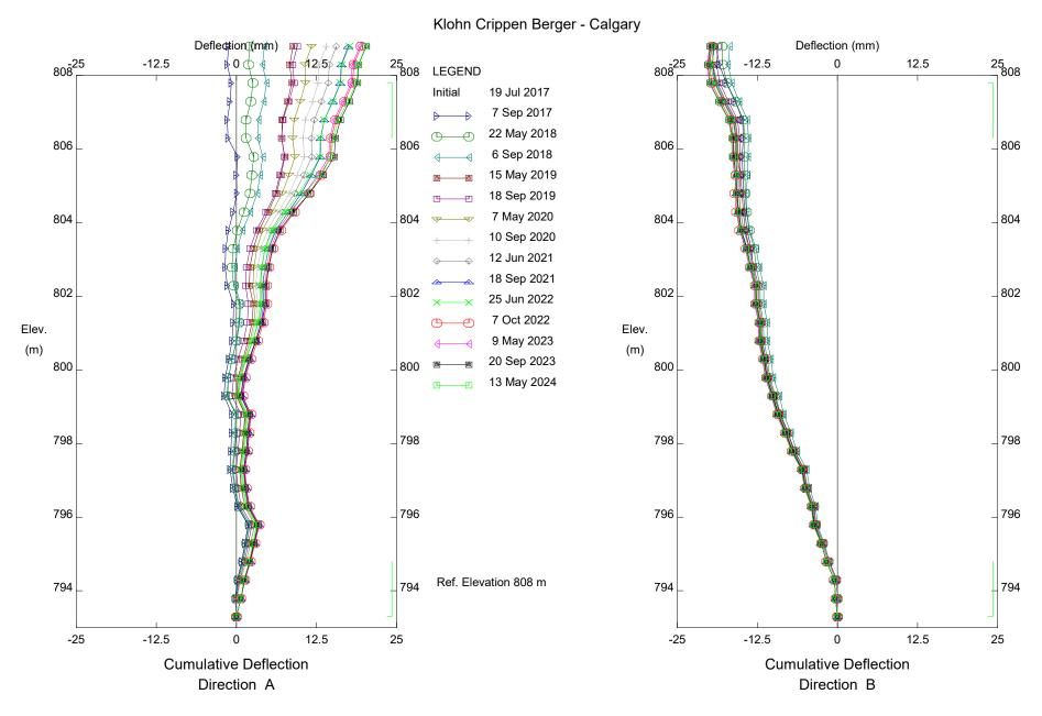
C067; H21:14, Kneehill Creek Slide, Inclinometer SI17-C67-03
