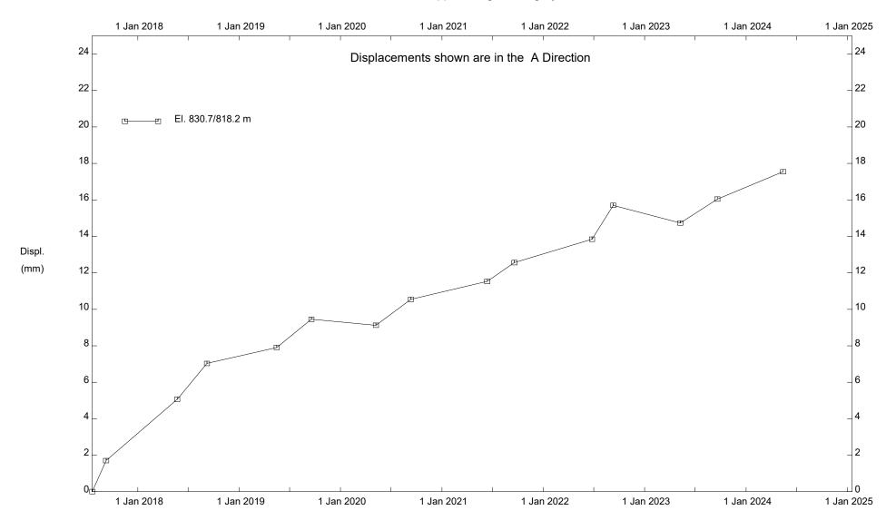
C067; H21:14, Kneehill Creek Slide, Inclinometer SI17-C67-02
