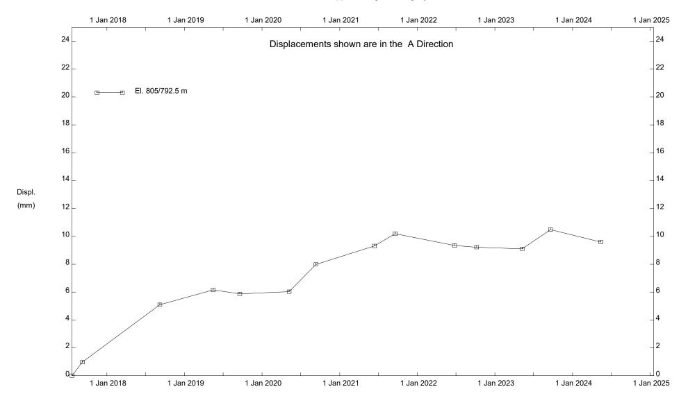
C067; H21:14, Kneehill Creek Slide, Inclinometer SI17-C67-05
