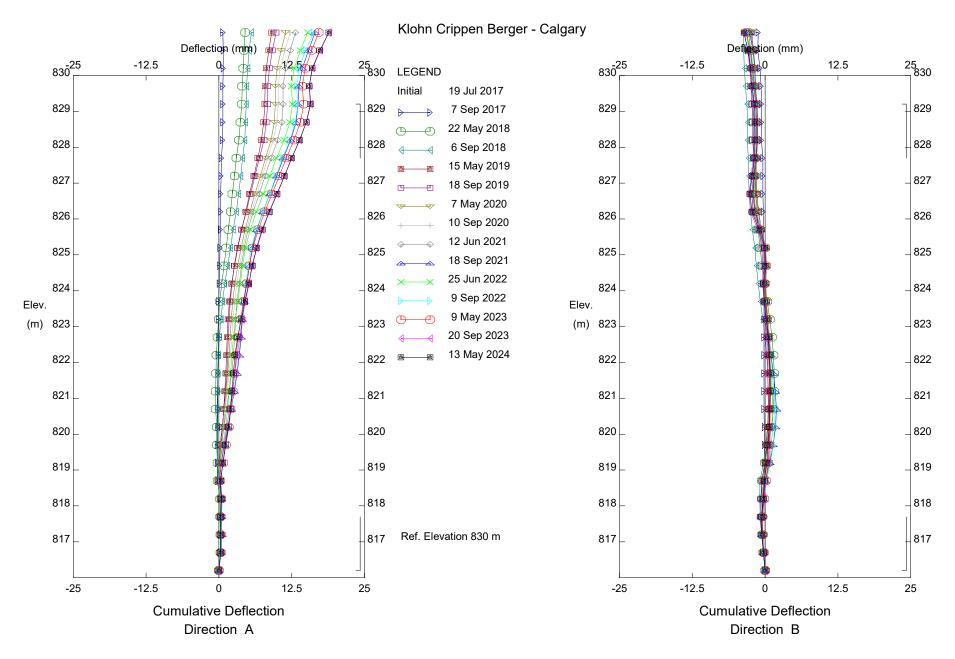
C067; H21:14, Kneehill Creek Slide, Inclinometer SI17-C67-01
