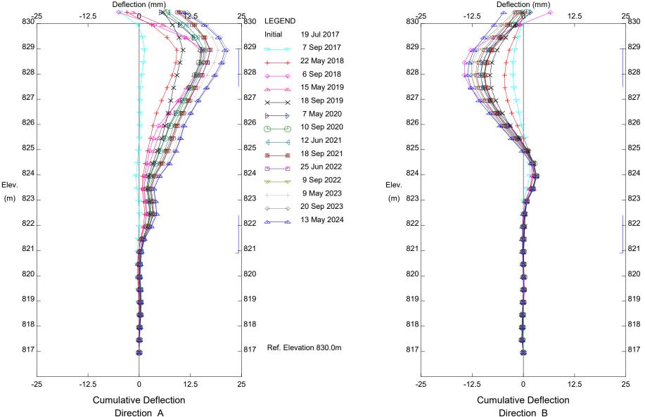
C067; H21:14, Kneehill Creek Slide, Inclinometer SI16-02
