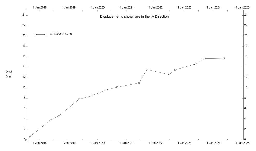
C067; H21:14, Kneehill Creek Slide, Inclinometer SI17-C67-01
