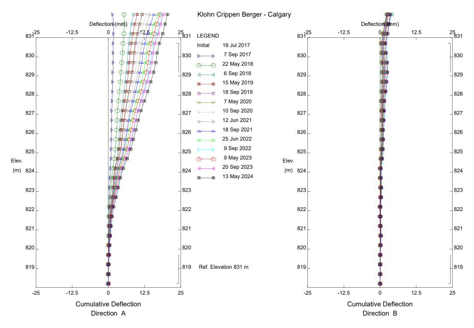
C067; H21:14, Kneehill Creek Slide, Inclinometer SI17-C67-02
