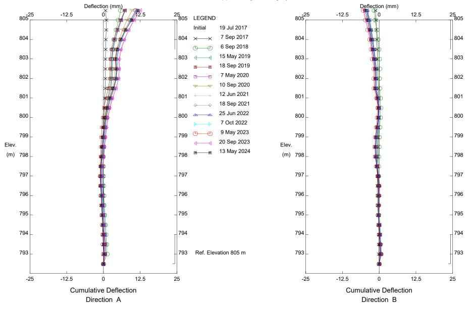
C067; H21:14, Kneehill Creek Slide, Inclinometer SI17-C67-05
