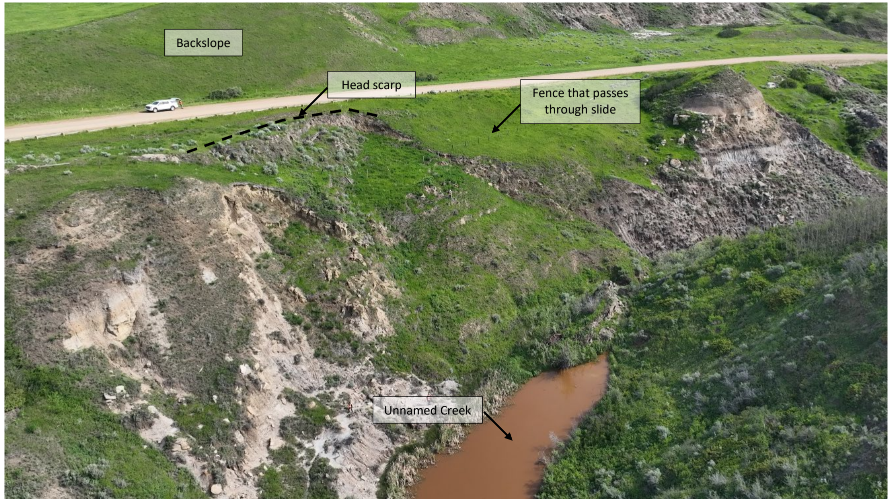
Photo 2 Oblique aerial photo of the C025 slide. Photo taken June 18, 2024, facing north-northeast.
