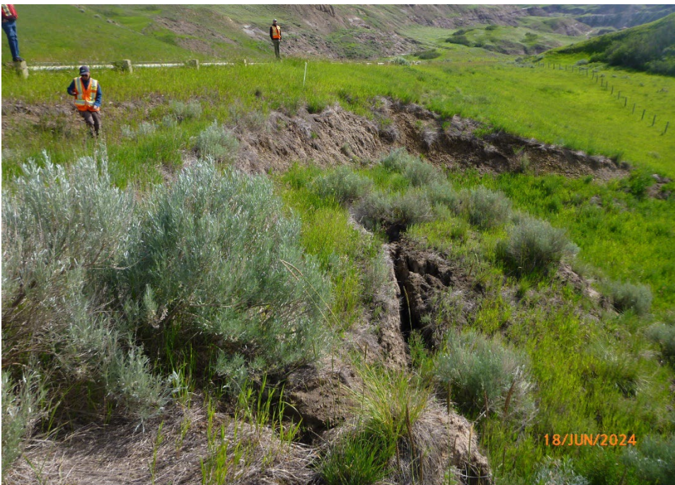
Photo 4 Head scarp of the slide where ground cracks were observed. Extent (number and width) of ground cracks have increased since the 2022 inspection. Photo taken June 18, 2024, facing east.
