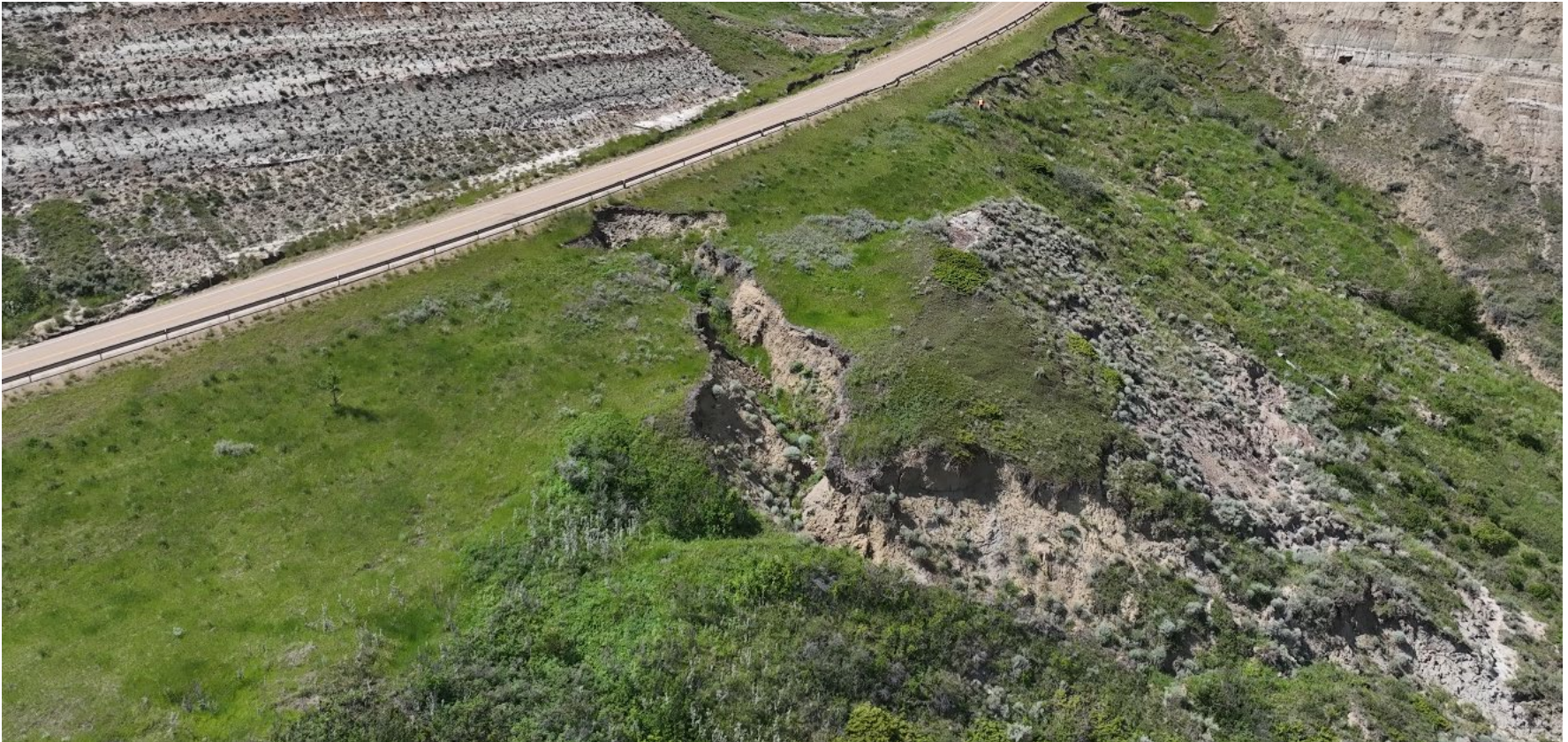
Photo 4 Aerial oblique photo of the C017-2 site. The degree of erosion appears to be similar as during the 2023 inspection. Photo taken June 18, 2024, facing southwest.
