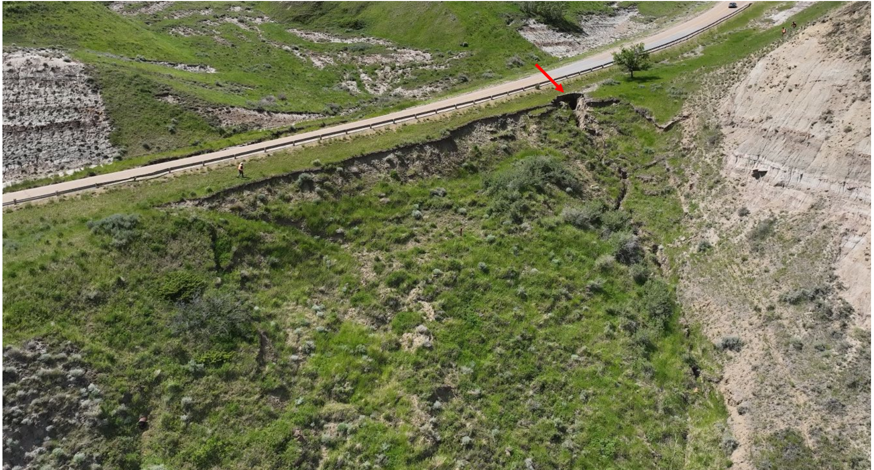
Photo 1 Aerial oblique photo of the C017-3 site. The slide appears to be in similar condition as during the 2023 inspection, but the amount of erosion of the west (left) side of the head scarp has increased (location indicated by red arrow). Photo taken June 18, 2024, facing southwest.
