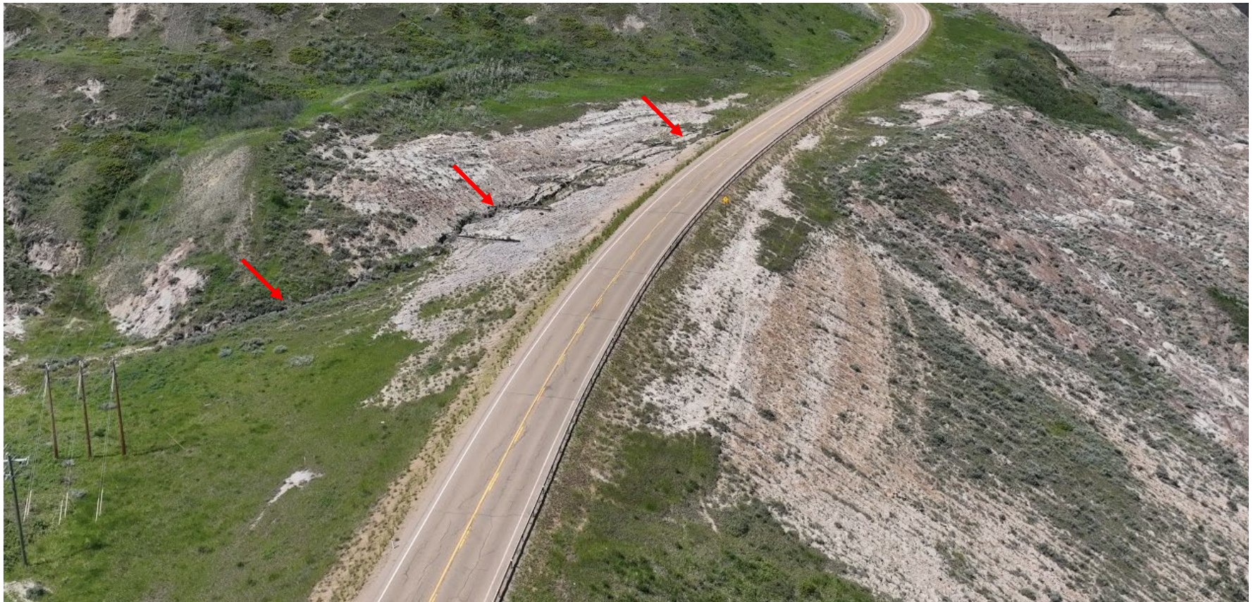
Photo 5 Aerial photo showing the east extent of the C017-2 site (ditch erosion indicated by red arrows) where the ditch grade increases to between approximately 15% and 20%. Photo taken June 18, 2024, facing west.
