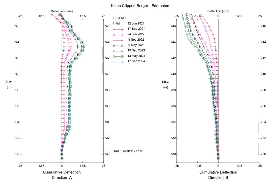
C017-III; H575:04; Truckstop Slide, Inclinometer SI20-01
