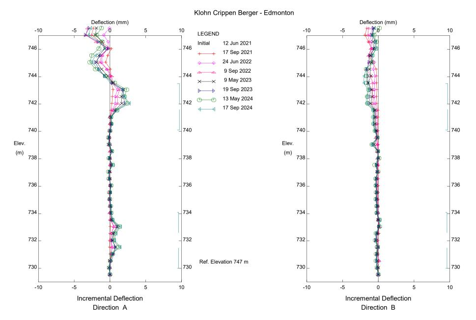
C017-III; H575:04; Truckstop Slide, Inclinometer SI20-01
