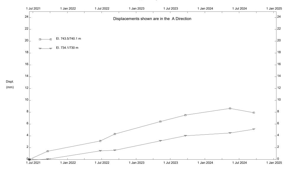
C017-III; H575:04; Truckstop Slide, Inclinometer SI20-01
