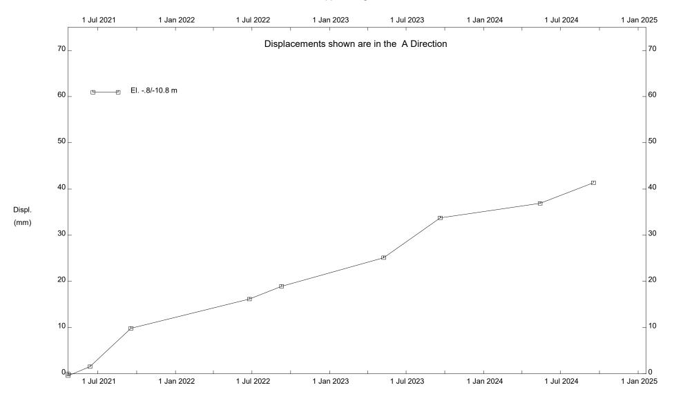
C048; H575:04; Slide W of Carbon Creek, Inclinometer SI21-C48-01
