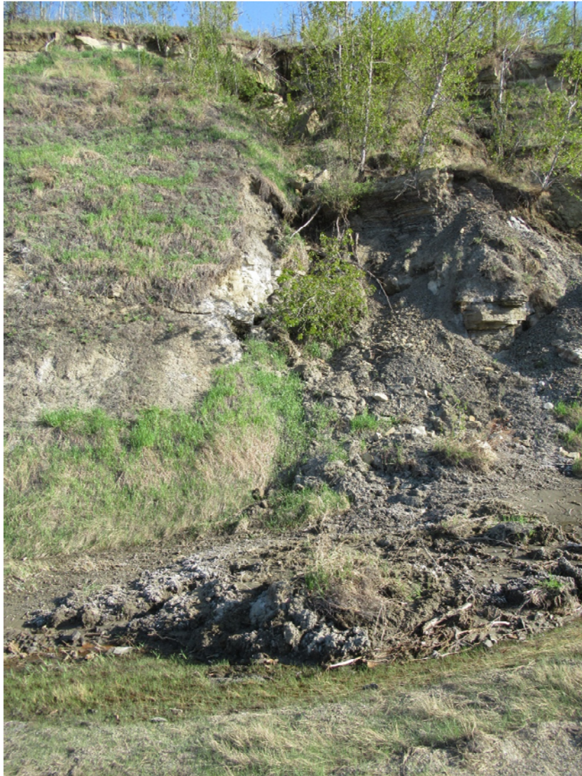
Photo 5: Looking north at gully at west end of debris flow with small fan of wet material at the base in the SBL ditch at km 12.415.
