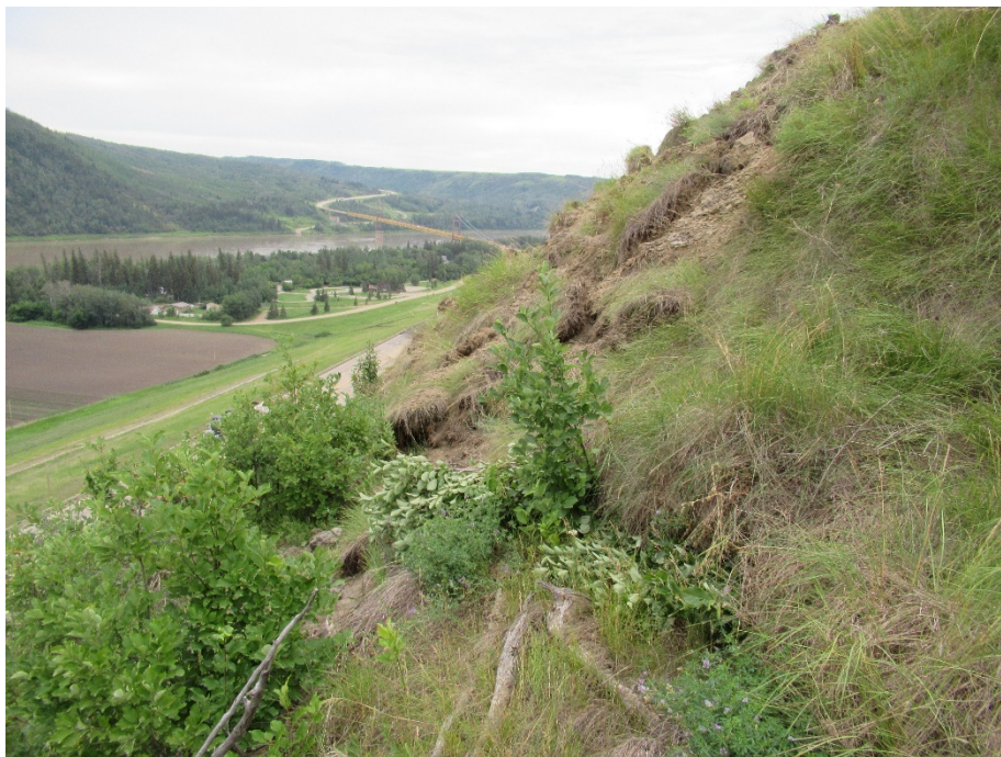
Photo 16: Looking west along the slide at the possible toe roll of the landslide (July 6, 2018)
