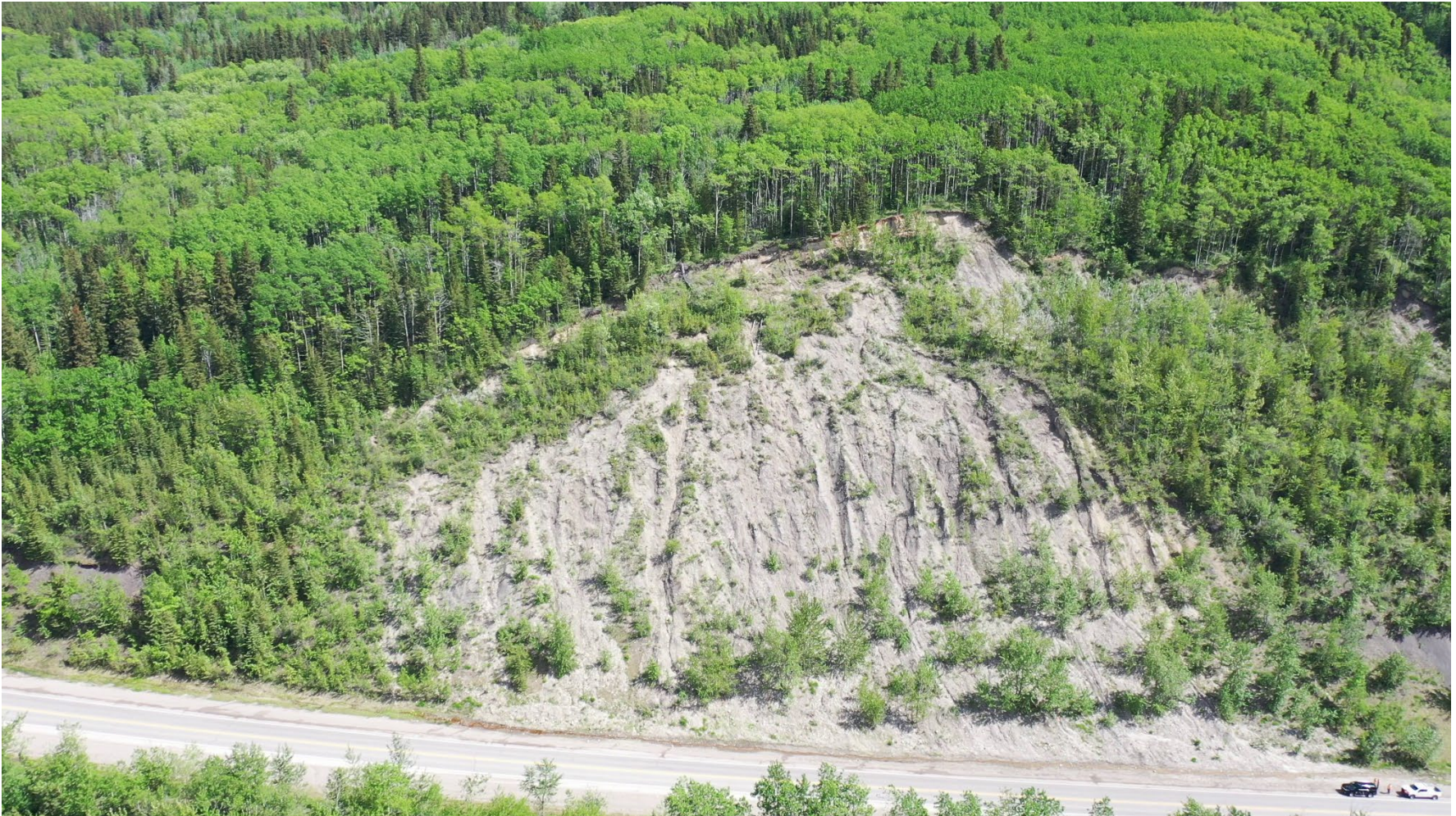
Photo 2 Overview of GP020-II site on Hwy 40:34. Note erosion gullies and poorly vegetated areas on backslope along east side of Hwy 40:34. Photo taken June 13, 2022, with UAV facing west.
