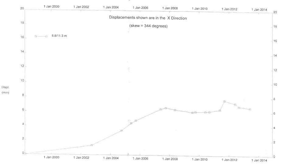
GP-6b; Sheep Creek Embankment, Inclinometer SI-03
