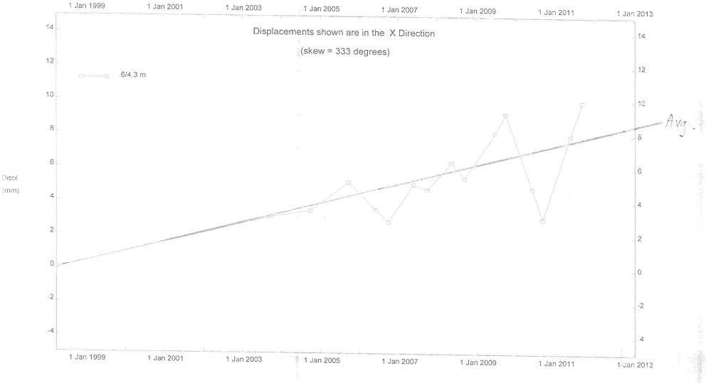
GP-6b; Sheep Creek Embankment, Inclinometer SI-04
