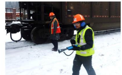
Figure 2: ULD cone-shaped direction sensor at CP's yard in Golden, B.C.
