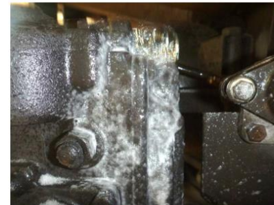
Figure 1: Example of soap and bubble testing of air brake components at CP's yard in Golden, B.C.
