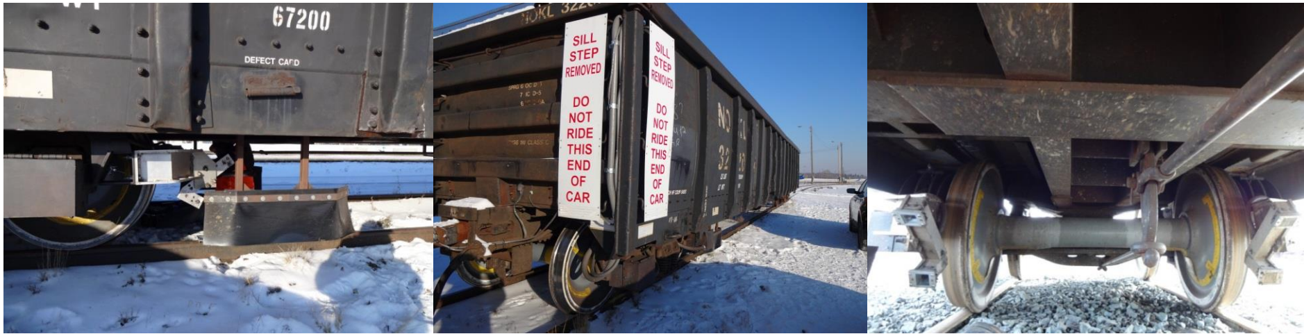
Fig. 6. Photographs of the CN and University of Alberta instrumented rail car (NOKL 322034) complete with a MRail / vertical track deflection (VTD) measurement system ( courtesy of A. Roghani, 2015 ).
